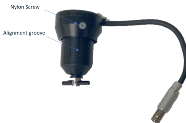
Figure 20: Stirrer assembly with nylon locating screw indicated.
